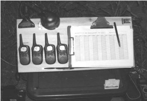
Photograph 2: Receiving station. Each receiver covered two radio detector locations simultaneously
